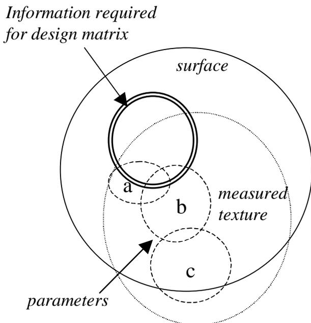
Figure 4. Information diagram, showing the information inherent in the texture. The solid circle represents the total information in the texture. The concentric circles indicate the information needed to make a correlation. The large dashed circle represents the information in the measured texture. The smaller dashed circles represent the texture characterization parameters. Parameters  $a$  and  $c$  are orthogonal
