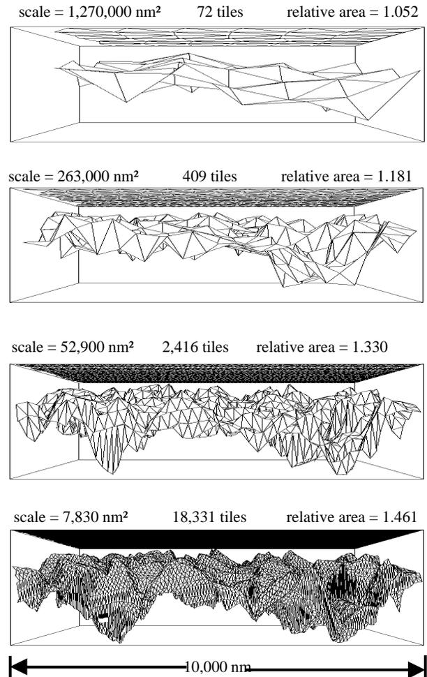
method on a measured surface. The scales of analysis, number of tiles and relative areas are given with the tilings. The diamond coating on a silicon substrate was measured by scanning tunneling microscopy at UNCC.
