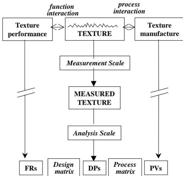
Figure 1. The three design domains for describing the texture in the physical domain, showing the importance of including the scales of interaction in the texture measurement and analysis.
