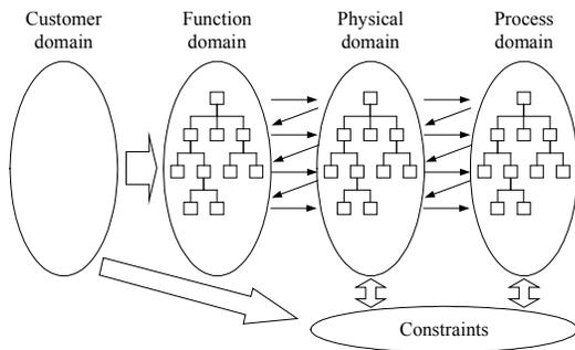
**Figure 2: The process model in Axiomatic Design**
