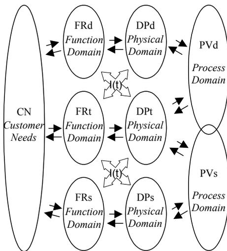
**Figure 9 The revised interaction model for design domains in an integrated synchronized environment for product development**
