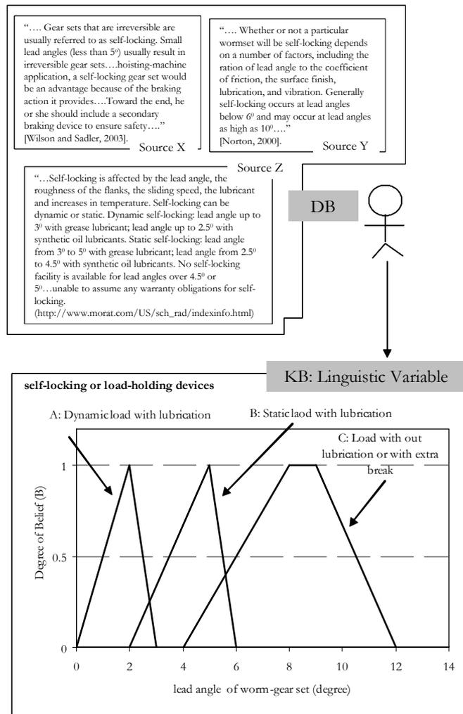
Figure 7. Linguistic variable for self-locking devices.
