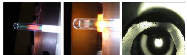
Figure 8. Behavior of the plasma inside the lamp (left) and the progression of pinhole failure (center). The sectional view of lamp shows internal state of pinhole failure (right).
