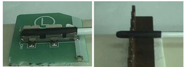
Figure 5. Clip type in LCD TV (left) and test bench (right) power electrode.
