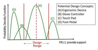
Figure 8. A common mistake of drawing probability density function curves.
