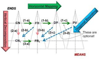
Figure 7. A "zigzagging" synthesis reasoning process [Lu and Liu, 2011].
