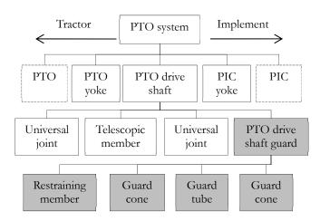
Figure 8. Decomposition of PTO system components.
