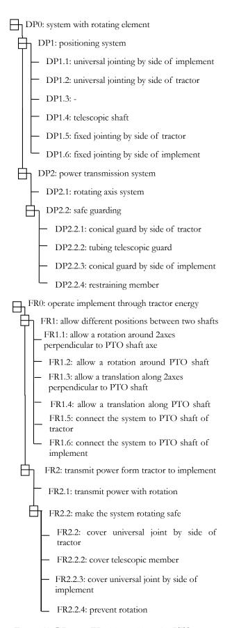
Figure 11. DPs and FRs hierarchies of a PTO system.
