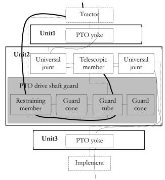
Figure 9. PTO system component interaction.
