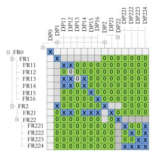
Figure 12. PTO system design matrix.
