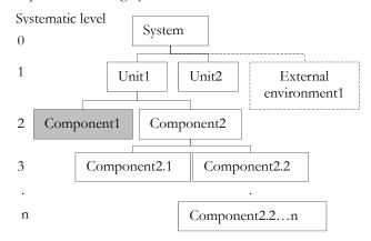
Figure 2. The product breakdown structure.
