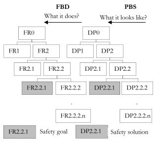
Figure 4. DPs and FRs hierarchy definition.
