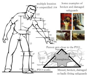
Figure 10. PTO system accident evaluation.
