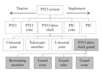
Figure 8. Decomposition of PTO system components.
