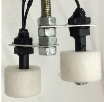
Fig. 5. Float switch configuration. The upper float is for fuel addition and the lower float signals emergency shutoff if triggered.
