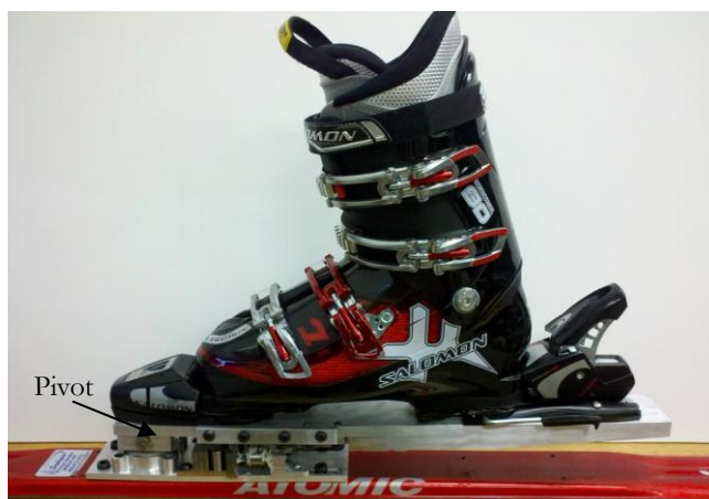
Figure 5. Group 3 final design [Austin et al. , 2011]. The pivot point is at the toe of the plate device. The plate rotates downward at the heel about this point.
