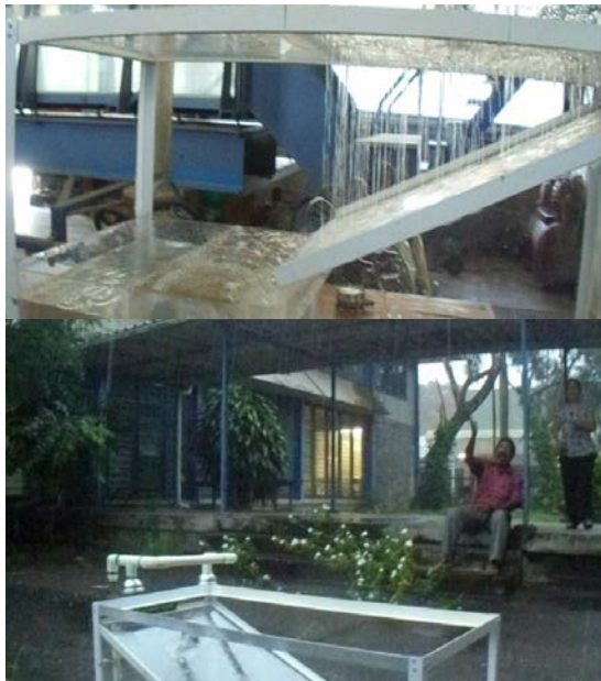
Fig. 8. (a) rainfall simulated from rain tray falling above the catchment; (b) rainfall captured outside
