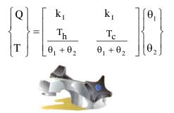
The above matrix equation is the transfer functions of the faucet. Per Equation (5), the [A] matrix is:
