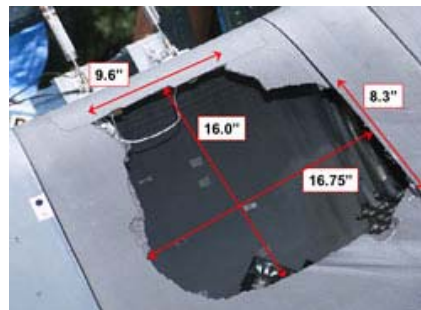
Figure 6: RCC impact test damage
