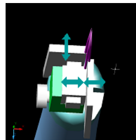
Figure 3. Design view to show actuating directions of each actuator in the gripper
