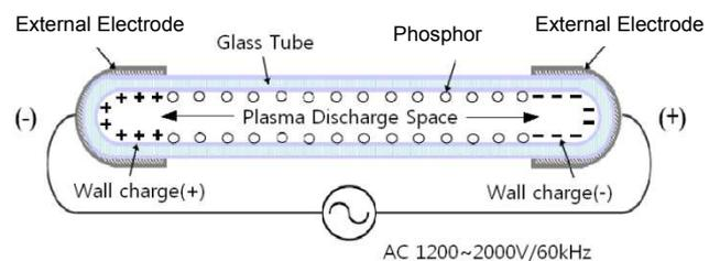
Figure 4. The operating mechanism of conventional EEFLs.
