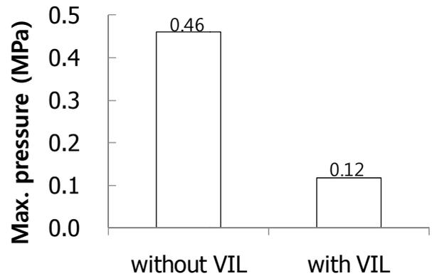
Figure 10. The impact test result with and without the vibration isolation layer (VIL).
