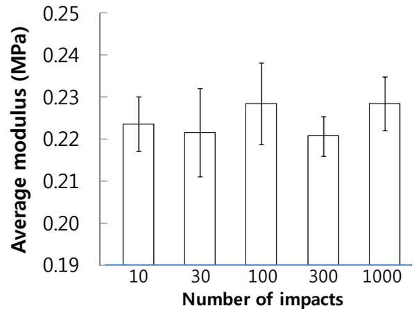
**Figure 7. The test result of impact fatigue test for glass wool mat.**
