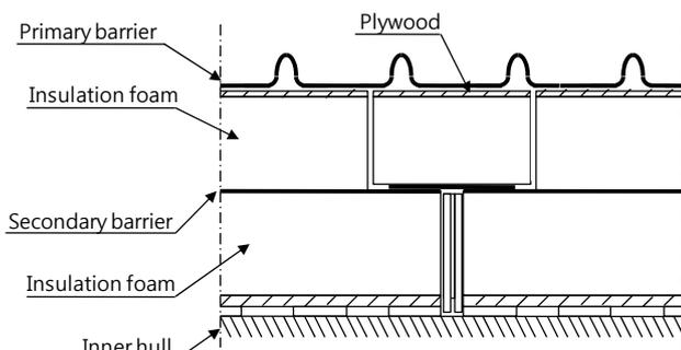
**Figure 1. Schematic diagram of configuration of membrane type LNG carrier.**
