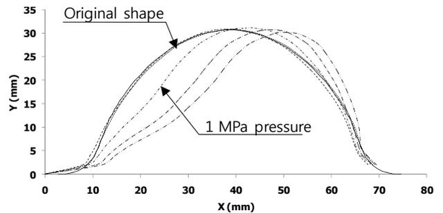
Figure 5. Experimental result of the corrugation shape after pressure is applied.
