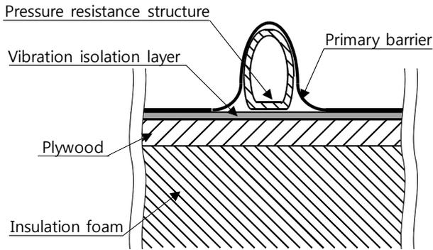
Figure 3. The schematic diagram of configuration of the vibration isolation layer.
