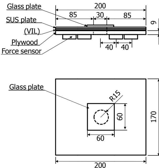
Figure 9. Schematic diagram of the specimen for the short duration impact test (unit : mm).
