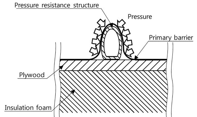
Figure 2. The schematic diagram of configuration of pressure resistance structure.
