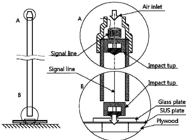
Figure 8. Schematic diagram of short duration impact test equipment.
