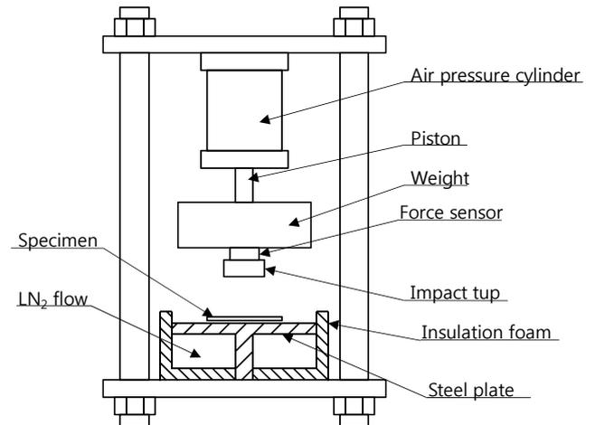
**Figure 6. A schematic diagram of low temperature impact fatigue test equipment.**
