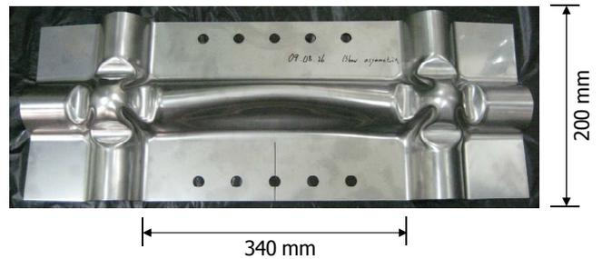
Figure 4. Specimen for pressure resistance test.
