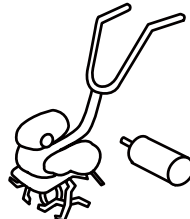
Rotary cultivator that runs with fuel from a gas cartridge for portable gas stoves
