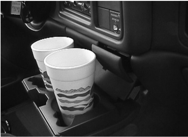
Figure 2 1999MY GM Silverado Cup-holders and Ashtray on Instrument Panel with Cups in Cup-holders
