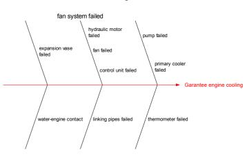
Figure 4 – Fishbone Diagram of the cooling system
