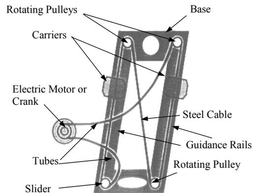
Figure 2. Integrated Dual-Cable Regulator
