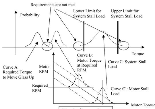
Figure 3. System Load Breakdown
