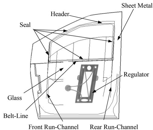
Figure 1. Typical Integrated Dual-Cable Glass Guidance System
