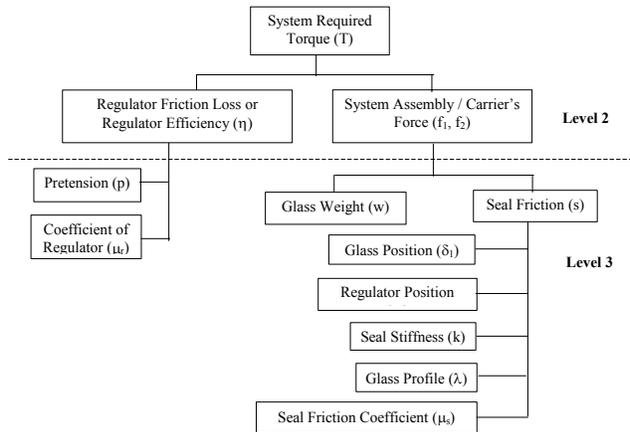
Figure 4. System Torque Hierarchy
