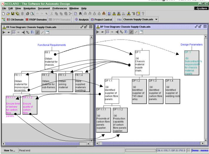
Figure 2. Car chassis supply chain FR and DP hierarchies defined in Acclaro software
