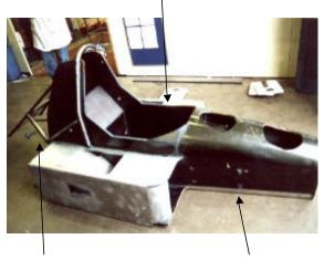
carbon fibre monocoque
