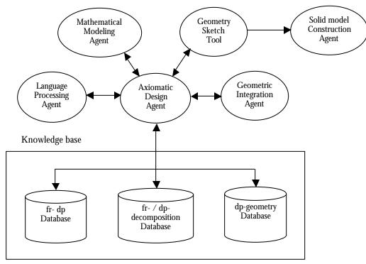
Figure 5. Proposed CAD system architecture
