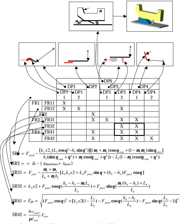
Figure 8. Links of FRs to system ranges and links of DPs to geometric entities on the design matrix
