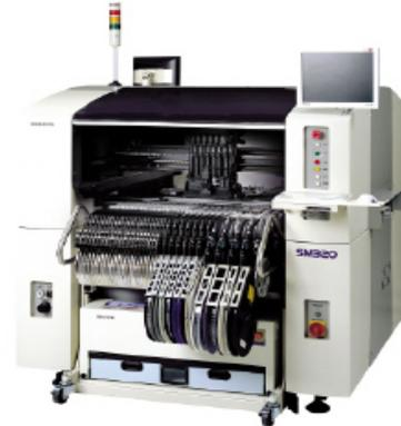
**Fig. 3** Chip mounter
