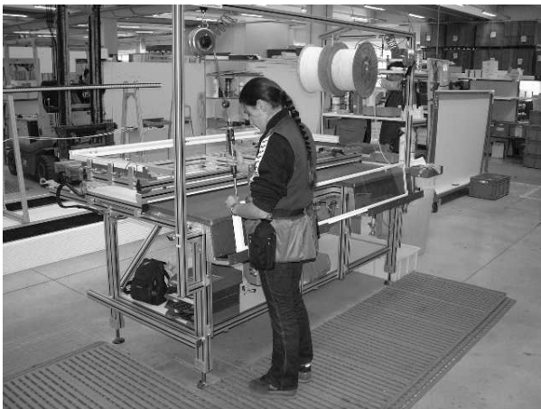
Figure 6: The new single-station manual assembly cell
