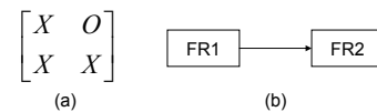
Figure 3. Design matrix represents design interaction structure and dictates a design process. (a) Decoupled design matrix (b) designing FR1-DP1 must precede FR2-DP2
