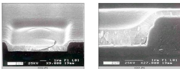
(a) cracking (b) thinning & high stress
