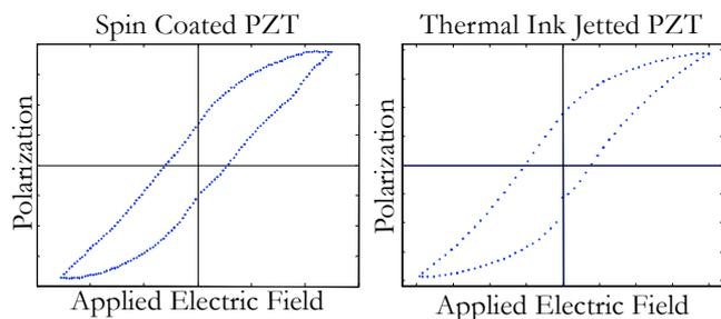
Figure 7. Polarization vs field tests for spin coated and printed PZT devices, units removed for comparison.
