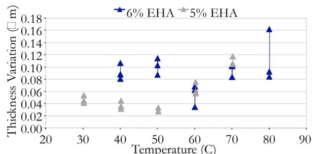
Figure 5. Thickness variation vs. substrate temperature for TIJed PZT on Pt.
