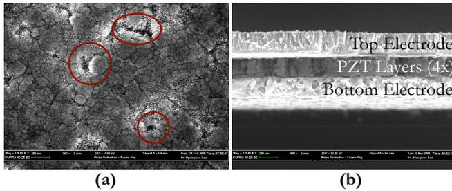
Figure 6. SEM images of (a) voids at PZT grain boundaries of a single PZT layer and (b) a multilayer film with no defects through the complete structure.
